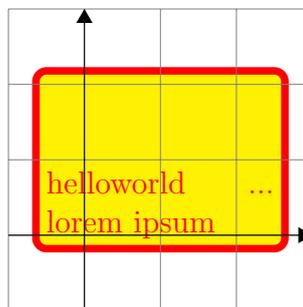
Note that the extra border (due to the inner sep) is beyond the specified width and height.
